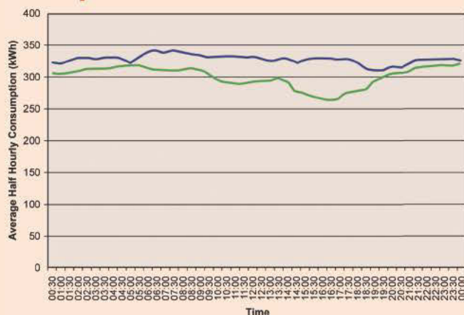
Figure 10 Average electricity consumption by half hourly periods pre and post installation of market-leading VO system
