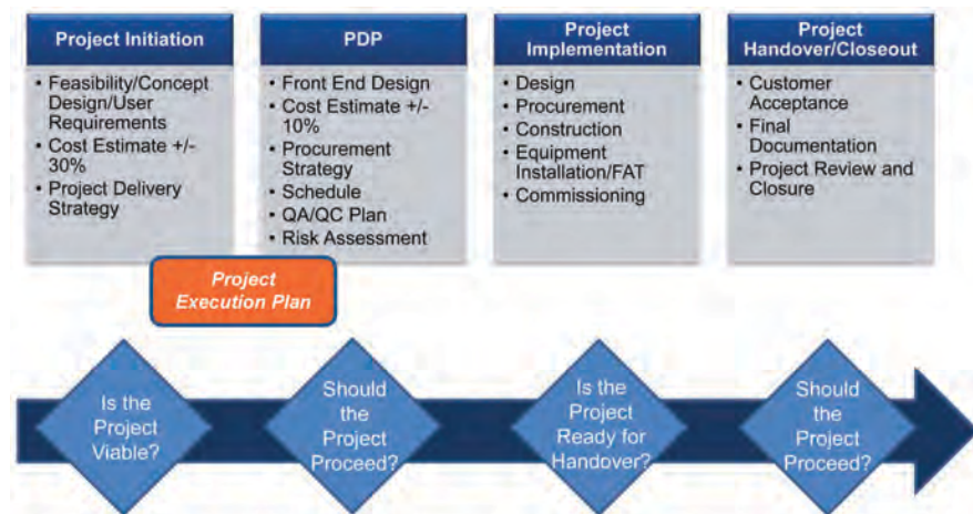
Figure 2. Key project execution activities – based on ISPE's Good Practice Guide: Project Management for the Pharmaceutical Industry project type matrix.
