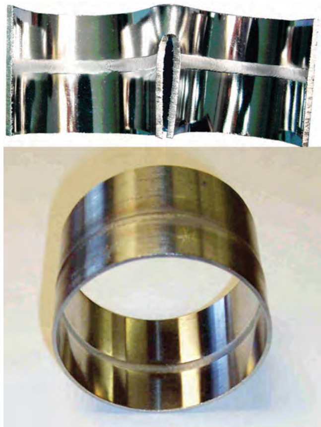
Figure 2. Top: An orbital weld coupon sectioned for visual examination of the I.D. surface for the semiconductor industry. Bottom: An orbital weld coupon made for the biotechnology industry. For High Purity Fluid Service, the welds must meet the acceptance criteria of the referencing code, i.e. BPE or SEMI and also meet the criteria in ASME B31.3 Table 341.3.2.
