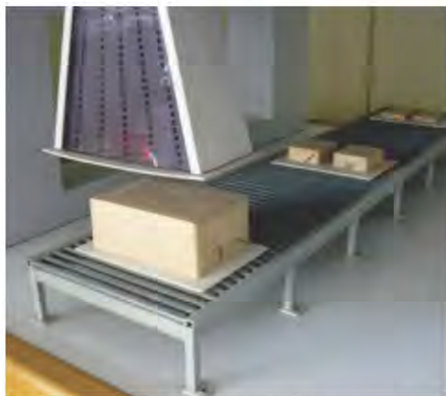
Figure 2. Materials passing under the e-beam scan horn (courtesy of Ion-Med, Spain).
