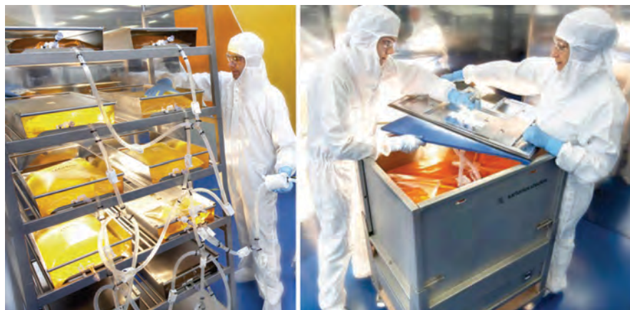
Figure 3. 2D-bags and 3D-bags for buffer storage, 2D-bags are installed on trays, 3D-bags are installed in pallettanks.
